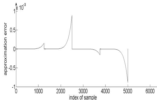
**Fig. 3. Approximation error of the sinus function generated by the: a) conventional NCO with Taylor series, b) novel NCO**
