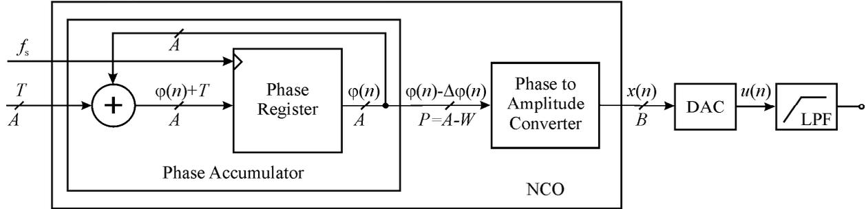
Fig.1. General block diagram of the Direct Digital Synthesizer
