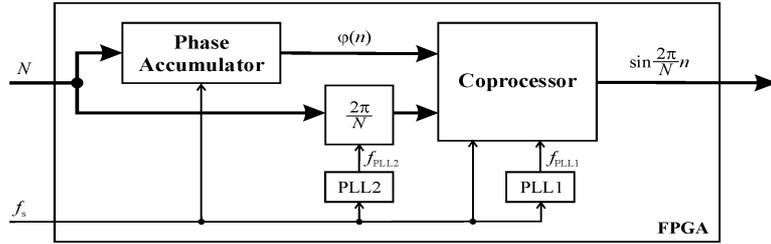
Fig.2. General block diagram of the proposed NCO
