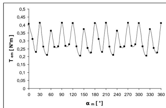
Fig.5. Electromagnetic torque of brushless DC motor as a function of angle of rotation.
