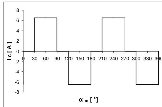
Fig.4. Current in phase C of brushless DC motor as a function of angle of rotation.
