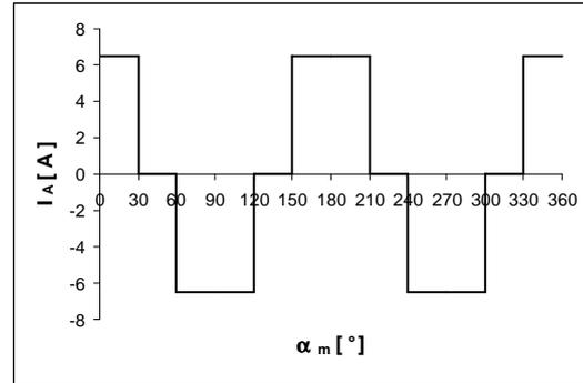
Fig.2. Current in phase A of brushless DC motor as a function of angle of rotation.
