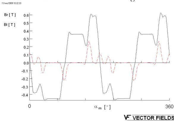
**Fig.6. Radial (continuous line) and tangential (dashed line) magnetic flux distribution of brushless DC motor in the air gap.**
