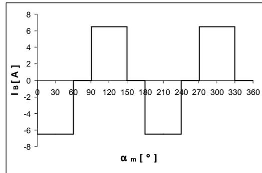
Fig.3. Current in phase B of brushless DC motor as a function of angle of rotation.
