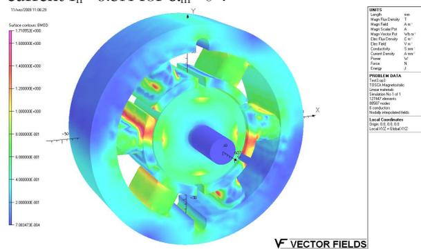
**Fig.7. Magnetic flux distribution in brushless DC motor;  $B_{max}=1.7 T$ .**
