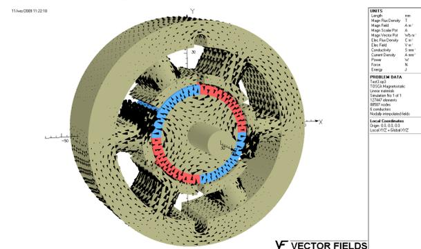
**Fig.8. Vectors of magnetic flux distribution in brushless DC motor.**
