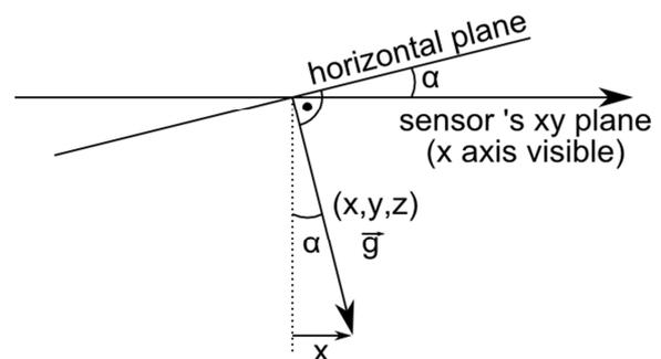
Figure 5. The g vector in sensor's coordinates
