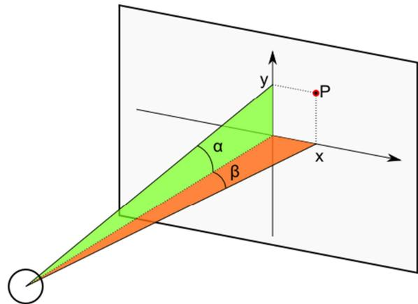
Figure 9. Spot projection on the screen
