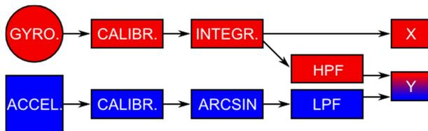
Figure 8. The Data Processing Scheme
