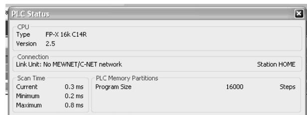
**Fig.4. Run parameters (scan time) for Panasonic FP-X C14R PLC**
