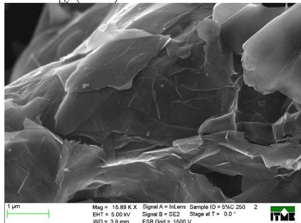
**Fig.1. SEM image of used Graphene Nanoplatelets (GNP's) material.**
