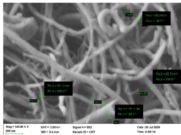
**Fig.2. SEM image of used Carbon Nanotubes (MWCNT) material.**
