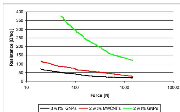
**Fig.7. Resistance changes under pressure on a logarithmic scale for the sensors 2 wt%, 3 wt% GNP's and 2 wt% MWCNT 's shown on fig. 3.**
