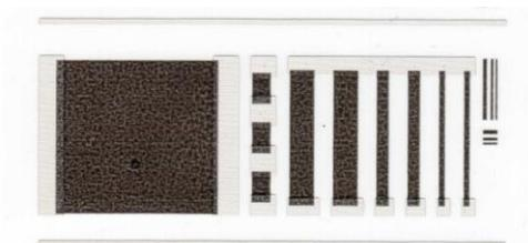
**Fig.5. Screen printed sample for electrical and mechanical tests.**
