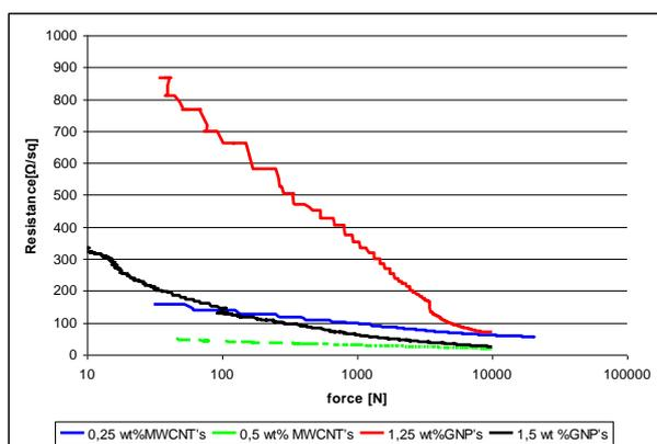
**Fig.7. Resistance changes under pressure on a logarithmic scale for the sensors 1,25 wt%, 1,5 wt% GNP's and 0,25 wt%, 0,5 wt% MWCNT 's shown on fig.4.**
